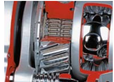
The oil deflector** ensures full lubrication of the power divider at very low vehicle speeds. Therefore, an oil pump is necessary only for special applications.
