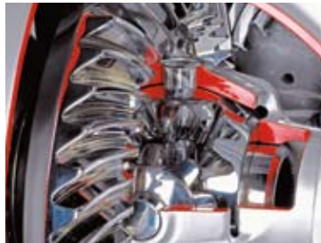
The differential case is half integrated in the ground wheel. Elimination of a pinion head bearing allows the use of a larger differential.
